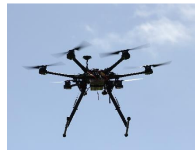
Multi-rotor UAV (hexacopter) surveying coastal environment.
