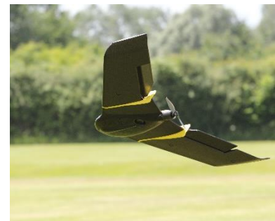
Sensefly eBee fixed wing mapping UAV with RTK positioning.
